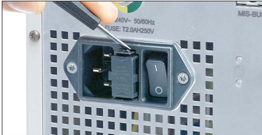
Figure 7-2: Releasing the fuse holder with a screwdriver.
