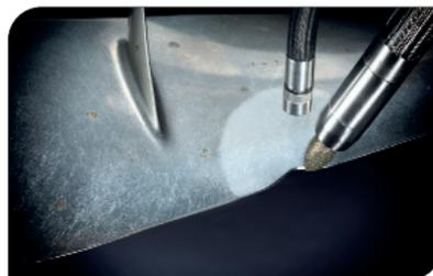
Removal of damaged material and turbine blade smoothing
