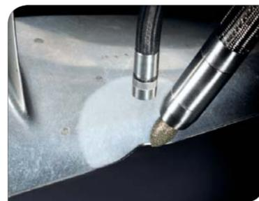
Removal of damaged material and turbine blade smoothing
