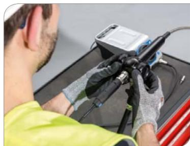
Precision control due to mechanical 1:1 gear ratio
