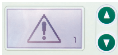
Figure 2-2: Message displayed on operating error in LED module.
