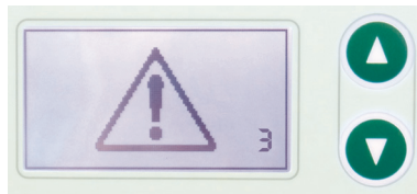
Figure 2-4: Warning displayed when temperature exceeds 60 °C.
