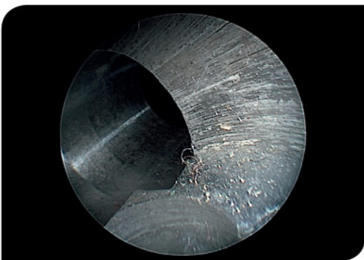
Inspection of drill holes to ensure they are free of burrs
