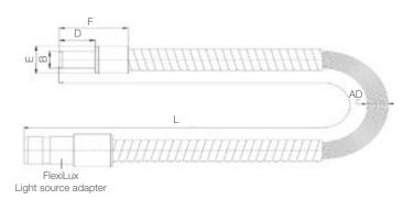
Very flexible due to covering with metal spiral hose and PVC coating
